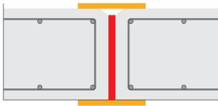
Where internal waterstops are used, correct fixing is essential to keep the waterstops in place during the concreting operations. Good compaction of the concrete around the waterstops is also necessary to avoid paths for water ingress.
